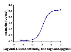
Immobilized Human LILRB2, mFc Tag at 0.5µg/ml (100µl/well) on the plate. Dose response curve for Anti-LILRB2 Antibody, hFc Tag with the EC50 of 13.0ng/ml determined by ELISA (QC Test).
